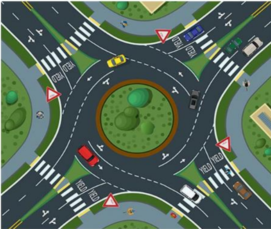
Illustration of a multi-lane roundabout. Source: FHWA
