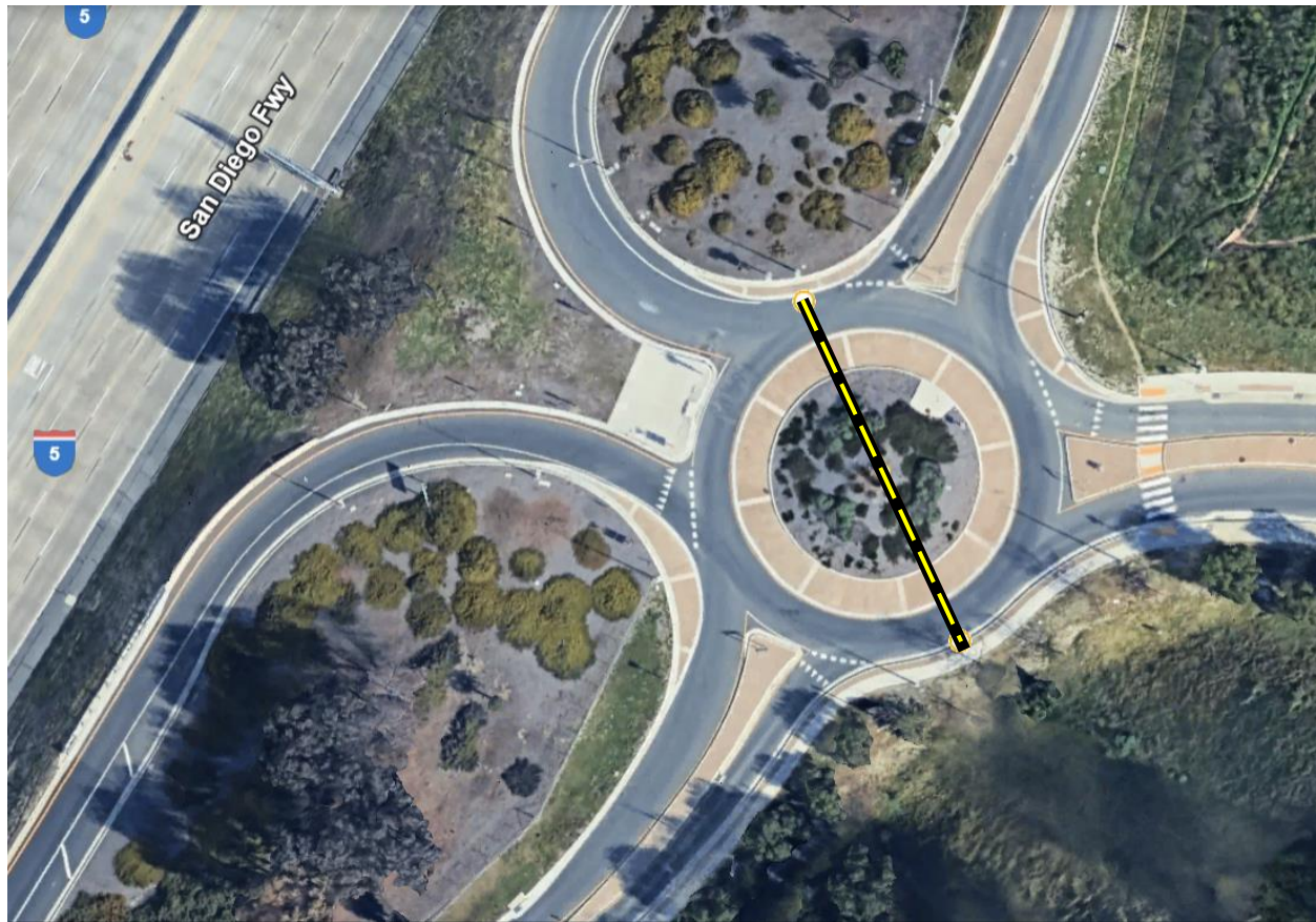
Conventional Roundabout at NB I-5 “hook” ramp terminal La Novia Road Interchange | San Juan Capistrano (D12)
