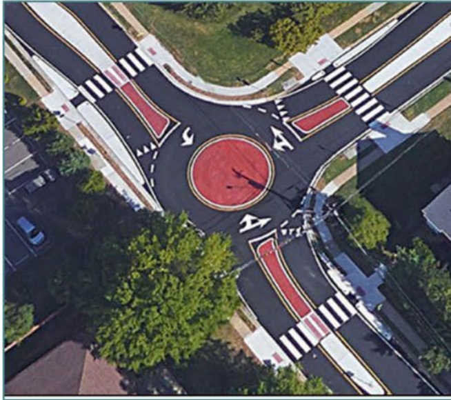
Mini-roundabout 48' to 90' (fully traversable)
