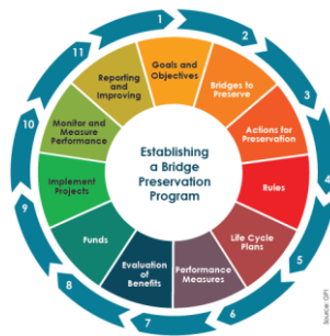
Figure 15. Steps for establishing a bridge preservation program.
